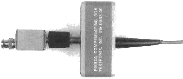
Figure 11-A4. The impedance matching box (extreme left) mated to the high voltage probe. Note direct connection. No cable is used.
